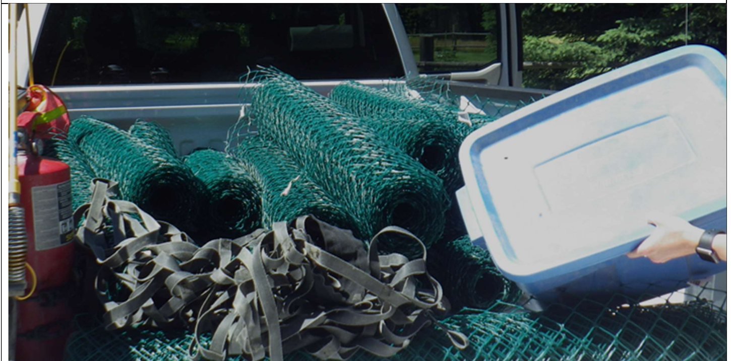
Photo 4. Spawning deterrent matting in rolls prior to installation in Swift Creek
