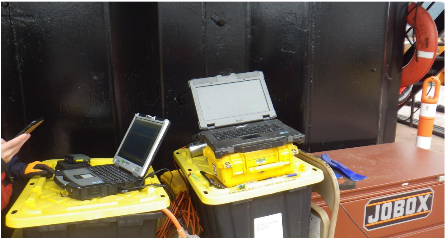
Photo 6. Computers used to record underwater noise levels measured by two hydrophones (one at mid-depth and one within two meters of the seafloor) during impact pile driving.
